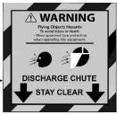
This sticker is located on the chip deflector on the back of the machine. When chipping wood, chips will be discharged out of the discharge chute at high rate of speed. Angle the discharge chute toward the ground to control the chips, and do not walk through the stream of chips while operating the machine.
