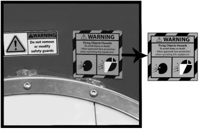
This sticker is located in the infeed chute. It states the requirement of eye protection, and a full-face shield is recommended. Wood flyouts may occur and the correct PPE will ensure that the operator is safe.
