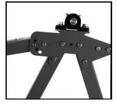
4. Find the Aluminum Reel Plate Assembly and slide the aluminum hub over the bearing shaft. The holes must be aligned between the aluminum bracket and main bearing shaft. Insert the bolt into the hole. (This fastens the Reel Plate to the Leg/Bearing Assembly.)
