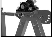
3. Find the Guide Arm, and remove the hinge bolt and retract the lock pin. Assemble the Guide Arm to the Bearing Mount and insert the hinge pin. (Do not tighten bolt. Bolt must only be snug). Then, add the nut to the bolt and lock the bolt. This keeps it from loosening while not over tightening the Guide Arm.
