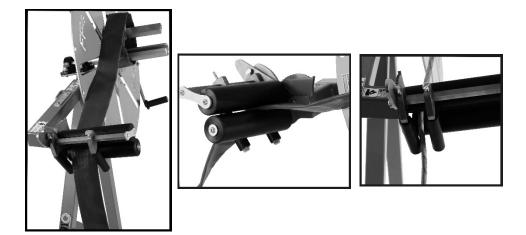
Use the ratchet action & thumbscrews to adjust the position of the guide rollers. Ratchet the horizontal rollers down to tighten. The vertical rollers should be at a 90 degree angle to the hose, rope or cord being wound and make sure it remains in the middle of the Fair Lead when winding. If the hose, cord or rope slips out of the Fair Lead stop turning the crank handle to prevent kinks and reset the material properly through the guide rollers.
