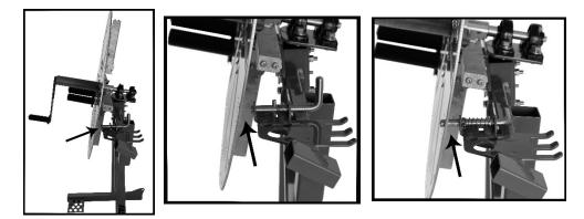
Remove the crank handle from its holder and insert it into the reel plate stem for turning the wheel.
