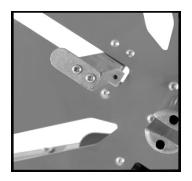
Take the lead end of the hose, cable or rope that is to be wound and secure it through the reel plate stem.
