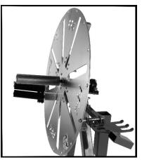
Use a large wrench or flat bar to tighten Main Reel Stem. Lock the Reel Plate with the lock arm, and slide the wrench or flat bar into the slot and tighten with 50 – 60 Lbs of force.
