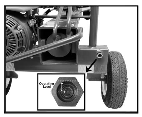
Oil Fill Level – Oil sight glass. Oil level must be sitting between the halfway and top of the sight glass. This means the reservoir is full and ready for operation.
